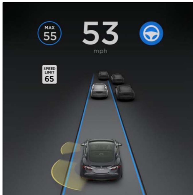
Figure 5. Autopilot User Interface showing System Perceived Lane Lines, Other Vehicles, and Ultrasonic Objects.
